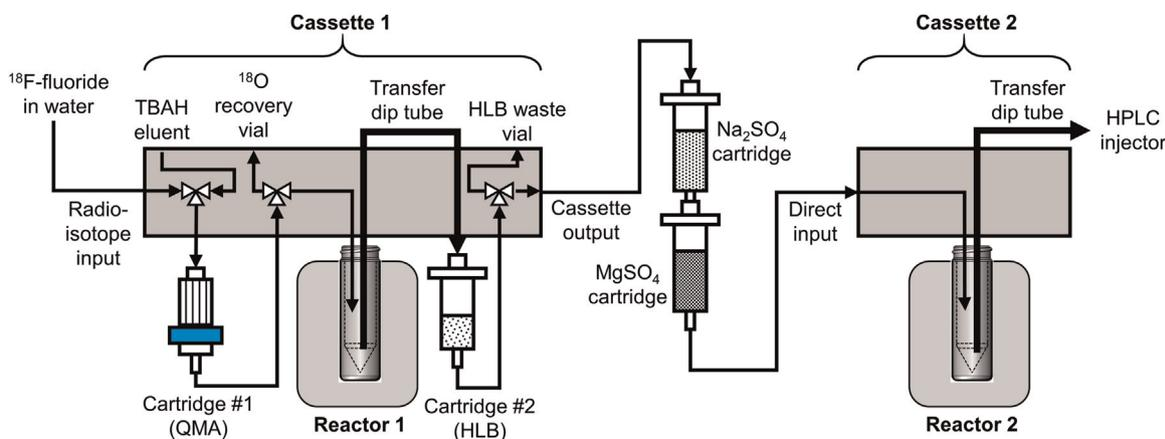
**Fig. 1.** Fluid diagram and cassette setup for automated  $^{18}\text{F}$ -FDHT synthesis. All components within the grey rectangles (i.e., three-way stopcock valves, transfer dip tubes, and the necessary fluid connection ports) are pre-installed in the disposable cassettes. Both cassettes are identical in construction and internal components, but unused components are omitted from Cassette 2 for clarity.
