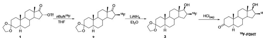
Scheme 1. Three-step synthesis of  $^{18}\text{F}$ -FDHT.
